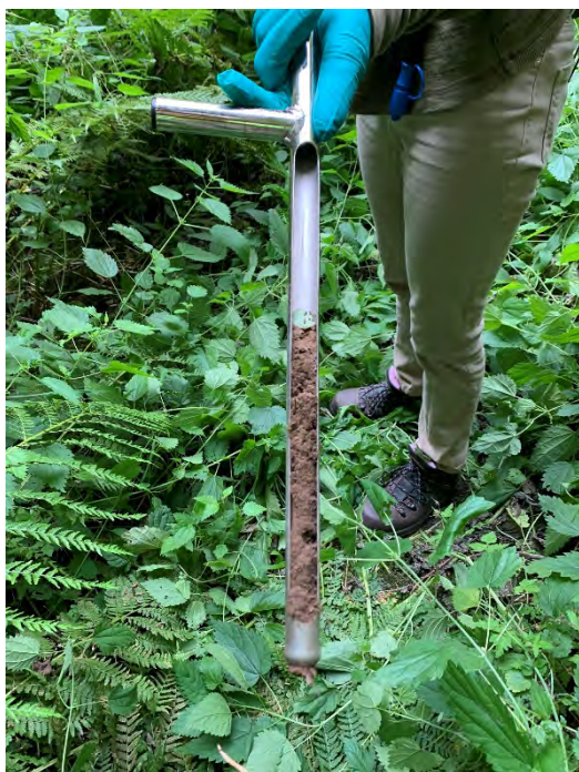
Photo 4. Soil core obtained from the push probe.
